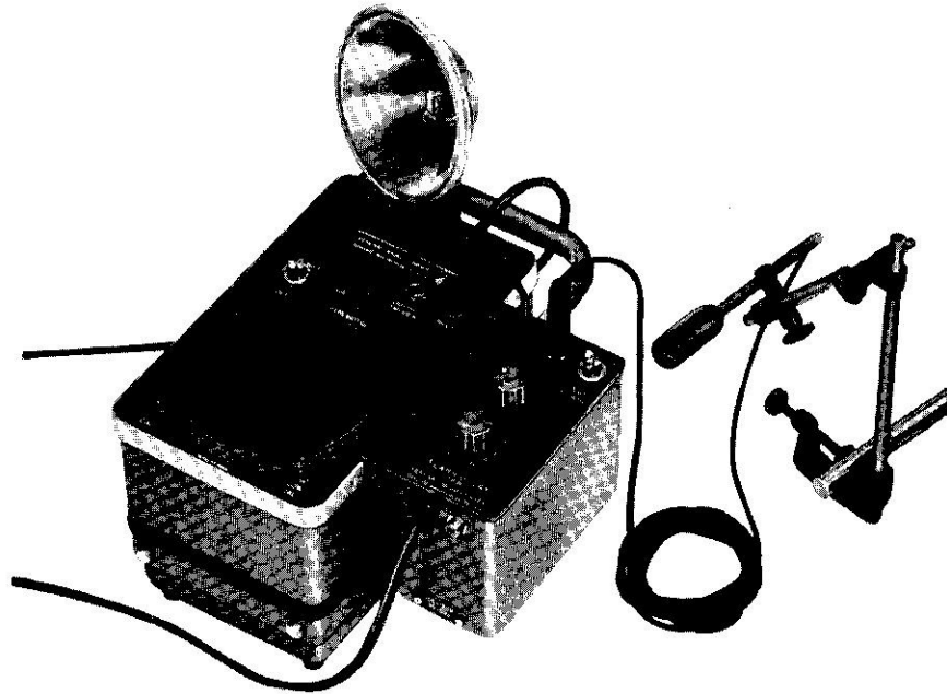
Figure 4-1. The combination of photoelectric pickoff, flash delay, and Strobotac or Stroboslave is all that is needed for most tachometric and motion-analysis applications.
